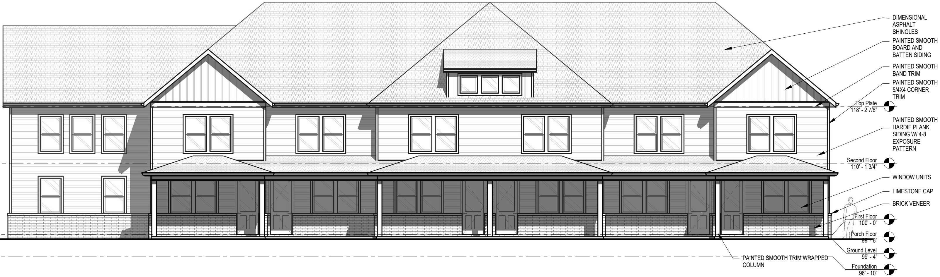
Building Elevation 1 Front/North 1/8" = 1'-0"
